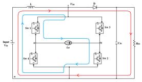
Fig 4: current flow diagram in power interval
