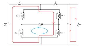
Fig 3: current flow diagram in shoot through interval
