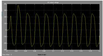
Fig 10: AC output voltage waveform with transformer for open loop BDHC
