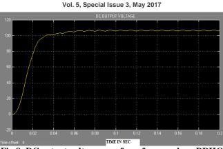
Fig 8: DC output voltage waveform for open loop BDHC
