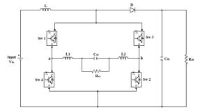
Fig 2: circuit diagram of BDHC.
