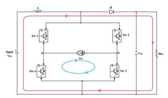
Fig 5: current flow diagram in zero interval
