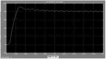
Fig 13: DC output voltage waveform for closed loop BDHC with reference voltage of 80V
