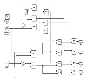
Fig 6: Simulink model for PWM generation circuit
