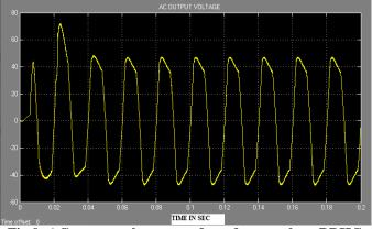
Fig 9: AC output voltage waveform for open loop BDHC
